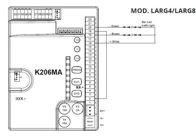
To connect traffic lights to a TAU boom gate with the 206MA control board connect your LED Traffic Lights as above with the negative from green to terminal 20 and the negative from red to terminal 18. positive for both green and red terminate at terminal 16. Also bridge terminals 2&19.
