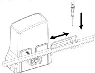
CAUTION The limit switch cams are used to operate the limit switches of the motor which, by means of the control unit, interrupt the movement of the gate during opening and closing. They must be positioned at the ends of the rack taking into account any inertia and the delay in stopping the gate with respect to the operation of the limit switches.
