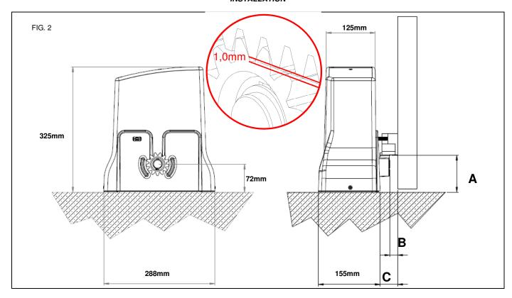
A = 105mm = VERTICAL DISTANCE BETWEEN THE TEETH OF THE RACK AND THE GROUND
